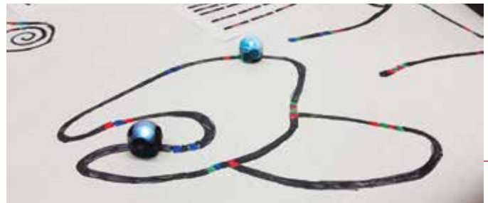
Self-propelled Ozobots run on a student-coded path.
